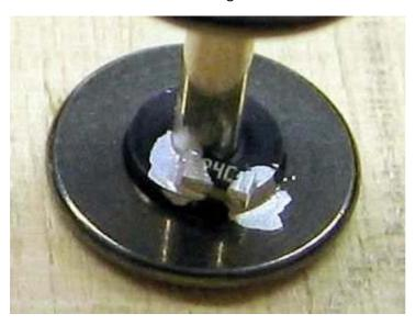
For double insulated axes (eg Fa. Luck), on the other side of wheel disc a connection between the axle and wheel disc to be established!
