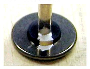
Now you should let the conductive paint to dry for some time. If you prepare a lot of wheels when you apply the silver conductive on SMD \*\*) till the last one probably the first prepared will be dry. Than then you can measure the wheels with Ohmmeter.
