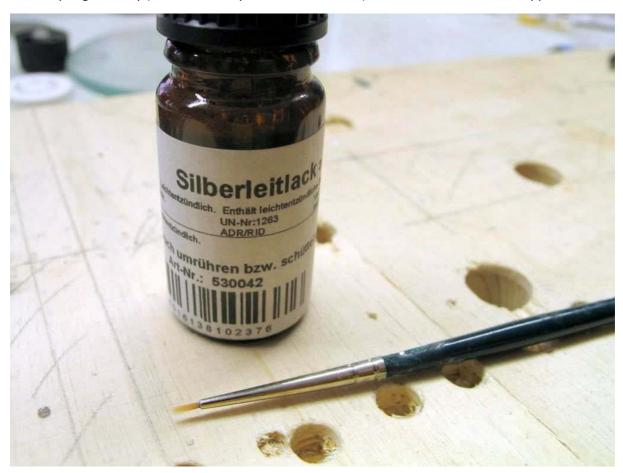
After having the conductive silver well shaken, taking a small amount with the brush (or toothpick) and establish a connection between the axle shaft and the contact surface of the SMD resistor that contacts the axle shaft. Then connects to the other side of the resistor with the wheel disk. You have to proceed this operation with some feeling and a steady hand in order to avoid a short circuit. For this operation I detach the axis of the wooden board and hold it in hand.
