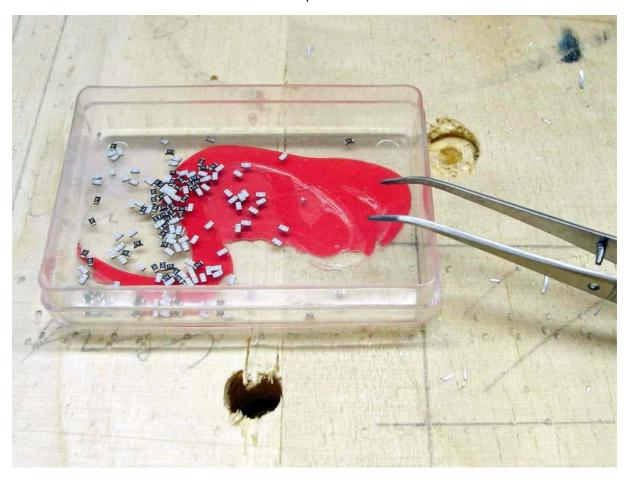
Put the drop of superglue on a smooth, dry, non-absorbent surface, ideally glass surface. Than with needle tip put small drops in the insulated part of the wheel. After install the SMD resistor and place it on the adhesive dots. Try to make contact between axes and contact surface of the SMD. No matter what visible side of SMD will be used. I prefer the black side.
