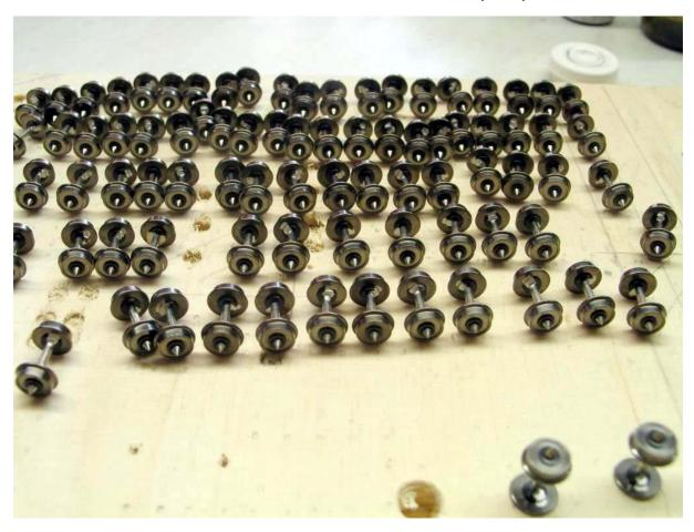
Last years Model Railway has started using PC based control and it requires detection of occupancy of tracks/lines. Therefore each passenger car/freight wagon should have two converted axis.
